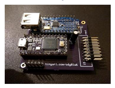
This keyboard modification allows open source Arduino parts to be used together in order to hook up a USB keyboard up to the TI-99/4A while the old keyboard is still attached and functional!
