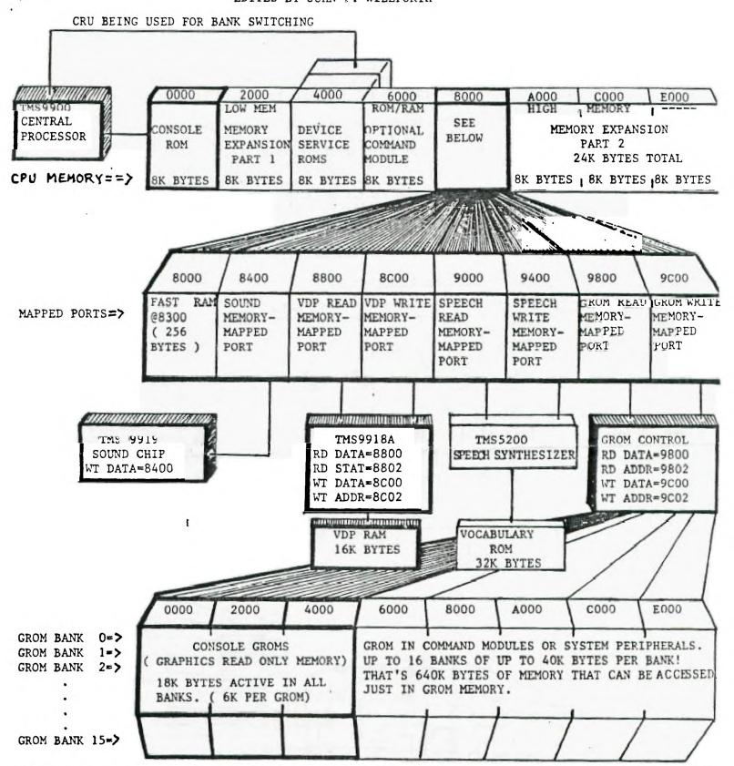
NOTE: THE HEAVY LINES INDICATE FEATURES INCLUDED WITHIN THE CONSOLE. I HOPE THAT THIS MAP WILL BE OF SOME USE IN CLEARING UP THE MEMORY SCHEME THAT WAS DEVELOPED BY TI TO MAKE MAXIMUM USE OF THE "GROM", AND THE ADDRESSING LIMITATIONS OF THE CPU (32K WORDS). FROM THIS DIAGRAM YOU CAN SEE, HOWEVER, THAT THE TI-99/4A HAS HAD THE POTENTIAL SINCE IT'S INCEPTION, TO BE A GREAT COMPUTING MACHINE.
