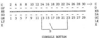
card, at the upper right of the console, pin 13 (LOAD) is the seventh pin from the left, on the bottom. is one end of your switch. Inside the speech synthesiser you will find that on the SAME side there are four tracks connected—11,12,13 and 14 from the left—this is the other end of your switch. For improved operation connect a 0.1mF by-pass capacitor across the switch and a 2.2k resistor in series with it.
