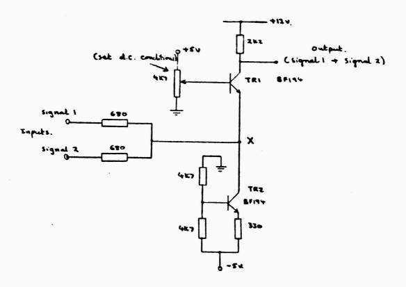
The summation of two voltages is accomplished at a low impedance (or 'virtual earth' point), so to prevent one input from 'seing' what the other input is doing.
