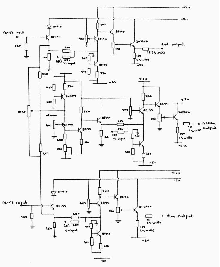
All resistors are  $\frac{1}{4}$  watt unless stated. Tolerance 10% Terminals marked (%) are luminance input from luminance amplifier. All resistor values are in ohms. e.g.  $560 = 560 \, \text{A}$ .  $2\text{K2} = 2,200 \, \text{R}$ .
