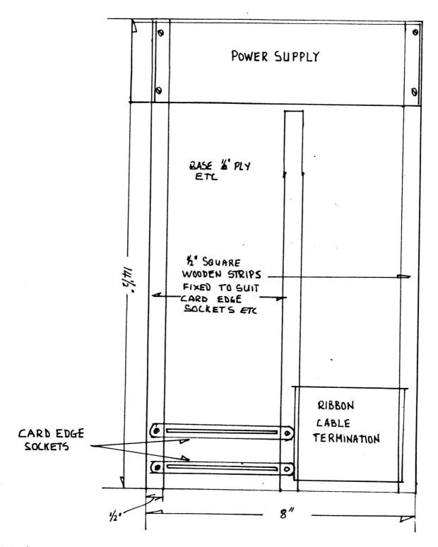
ALL SOCKET CONNECTIONS HARD WIRED BACK TO RIBBON CABLE TERMINATION AS ORIGINAL BOX WIRING: KEEP MAINS AWAY FROM COMPUTER WIRING!
