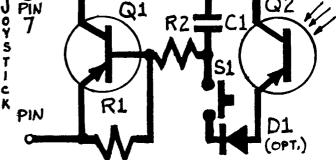
Acquire a large felt tip pen to use as a housing for the above aparatus. An old joystick cable will make a perfect cable with the female 9-PIN D TYPE connector, which will make assembly easier, faster, and definitly more economical.
