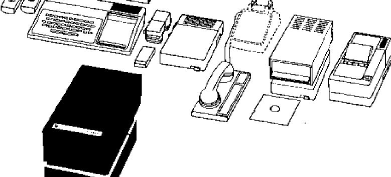
The Texas Instruments Disk Memory Drive is a minifloppy disk mass storage system with a 1 to 3-disk memory drive capability. Use of the Ti Disk Memory Drive requires the TI-99/4 Disk Drive Controller (Model PHP 1800).
